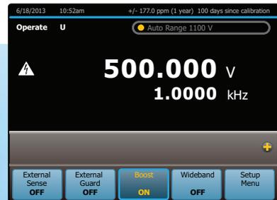
Product features like Boost and Wideband are easily activated via the five-button toolbar located at the bottom of the output screen.
